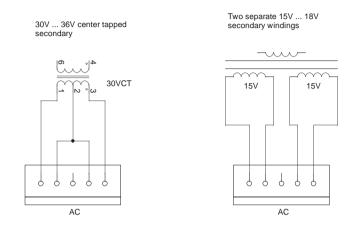
primary / mains voltage side not shown. Only work with mains voltage when you are qualified - then you know how to connect fuses, switches, earth GND etc. as well. If not, let some qualified person do it, or use a wall wart instead.
